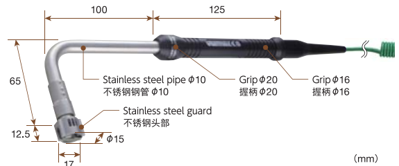
Type K K型热电偶 Model SX-173K-01-1-TPC1-ANP Type E E型热电偶 Model SX-173E-01-1-TPC1-ANP
