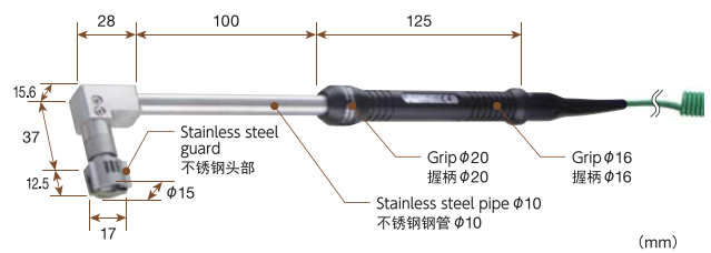
Type K K型热电偶 Model SX-174K-01-1-TPC1-ANP Type E E型热电偶 Model SX-174E-01-1-TPC1-ANP
